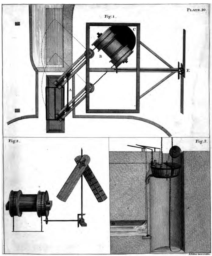
Fig. 1. Plan of the . Machinery with the mode of heeping the Craines parellel by the Lever A.
